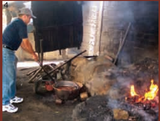
Quenching the copper in cool water after pulling it out of the red-hot fire. This creates the gorgeous variation in color and strengthens the structural properties of the metal.
