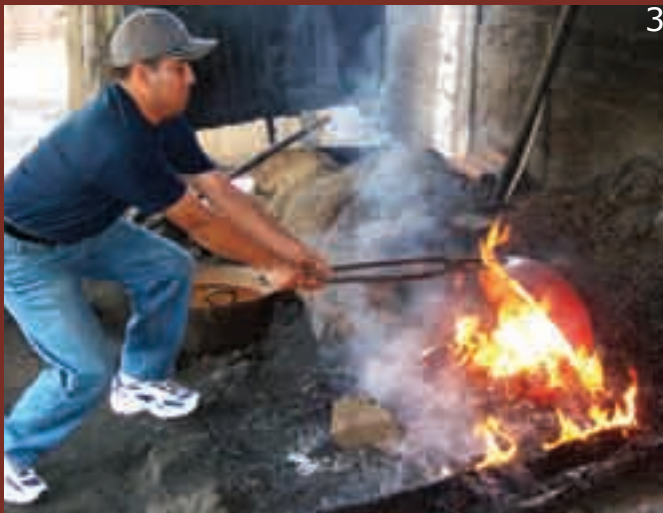
The Annealing Process (heat treating/softening the metal after it has been work hardened with steel tools).
